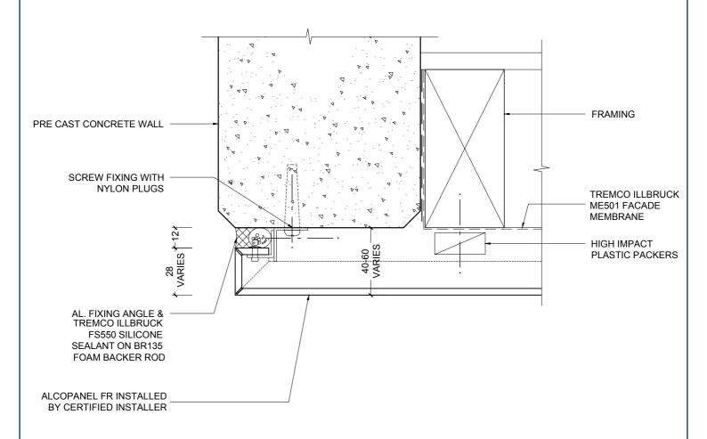
1 DETAIL AT PRE CAST CONCRETE WALL
